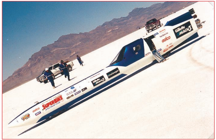
Richard Brown's 350mph rocket-powered motorcycle streamliner
