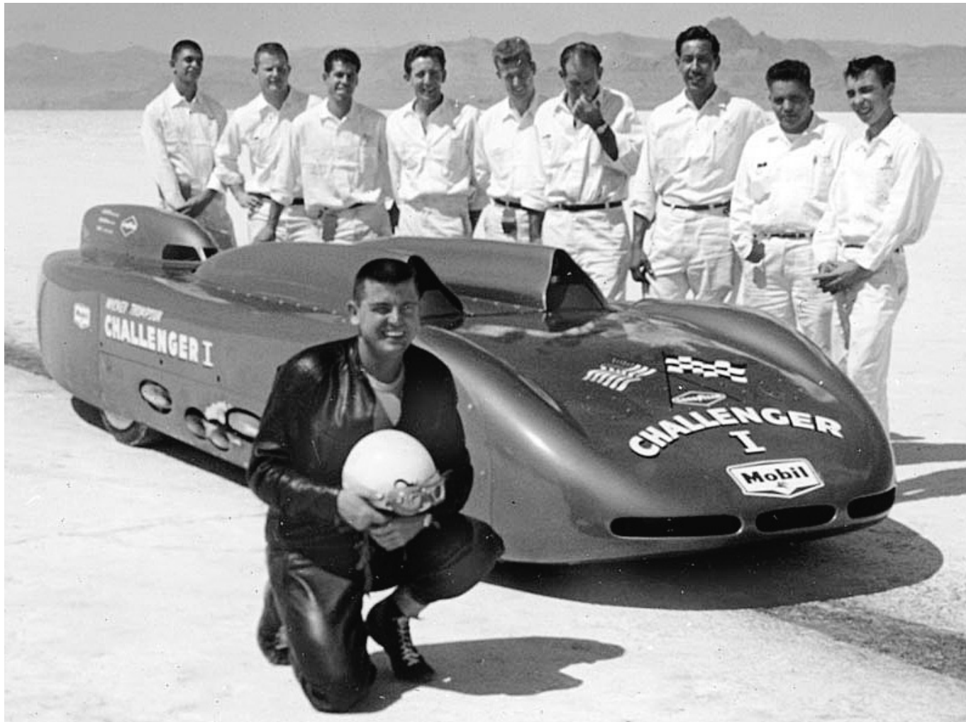
In his younger, wonder days, Mickey Thompson and crew were all smiles on the salt. The car exceeded 400MPH, only the second one in history to do so (Britain's John Cobb was first) and the first American. Unfortunately, on the 406MPH run the drive-shaft broke dashing Thompson's hopes for a world record as repairs could not be made within the slim 60 minute turn-around window.
